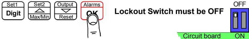
Press briefly to view each existing setpoint, if one has already been set. The LEDs to the right of the display will illuminate to show you which alarm channel you are viewing.
