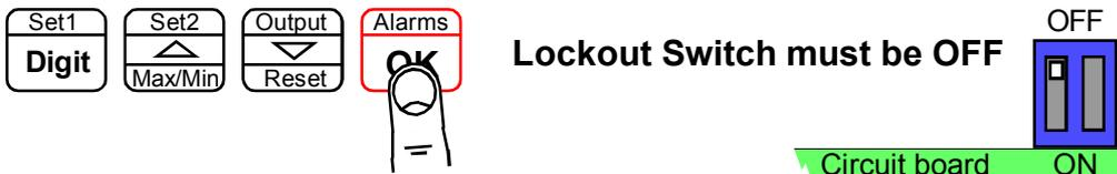
The diagram shows a control panel with four buttons: 'Set1 Digit', 'Set2 Max/Min', 'Output Reset', and 'Alarms OK'. The 'Alarms OK' button is highlighted with a red box. To the right, a 'Lockout Switch' is shown in the 'OFF' position. Below the buttons, a green bar indicates 'Circuit board ON'. The main display shows six red digits, all of which are dimmed.
