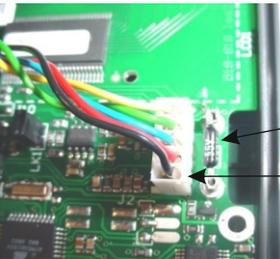
Shunt calibration resistor
