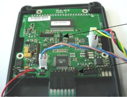
Sensitivity link should be in position for use with sensors, with sensitivities  $\leq \pm 5\text{mV/V}$
